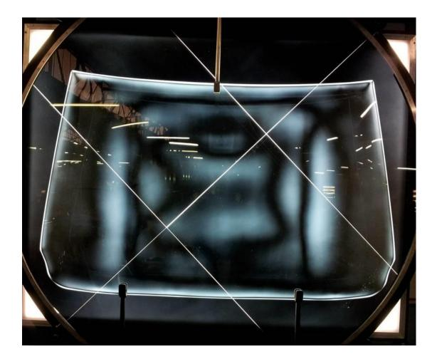
The second defect, "induced stress" is additional stress added to the already weak area when the windshield is installed into the vehicle body. The added stress is enough that when an object, such as a pebble, hits this weakened area during the windshield's normal, intended and foreseeable use, it can cause a pinhead size fracture to crack to over 130 mm in length almost immediately. These cracks cannot be repaired to the original windscreens structural integrity.
